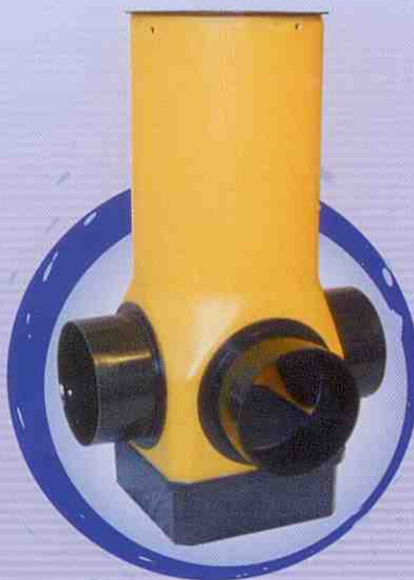
Drainage chamber "Conflur" DN 300 high 800 mm, 3 inlets
